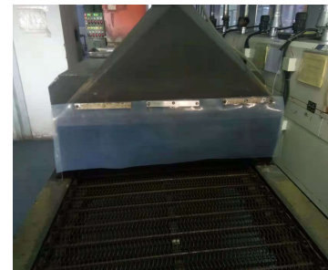
TAIPAQ Plant tunnel oven replacement of windshield strip before/after improvement
