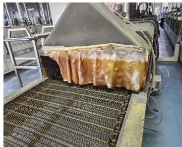
TAIPAQ Plant tunnel oven replacement of windshield strip before/after improvement
